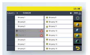
Up to 16 binary feed, ejection, and coil end sensors are visualized and monitored in an overview mask.
